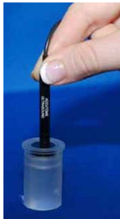
Figure 9.6 - Using the A-Scan Test Block
